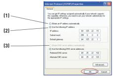
5. If "Use the following IP address" (2) is selected, your Modem/Router will need to be set up for a static IP connection type. Write the address information in the table below. You will need to enter this information into the Modem/Router.
